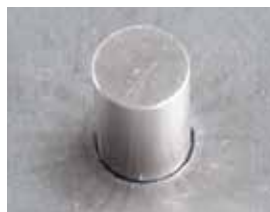
12 mm (1/2") hole cut with True Hole technology
