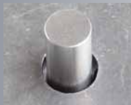
12 mm (1/2") hole cut without True Hole technology
